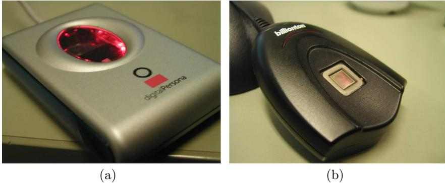
Figure 1: Our sensors — (a) Digital Persona U.Are.U 4000 (b) Billionton capacitive fingerprint reader.
