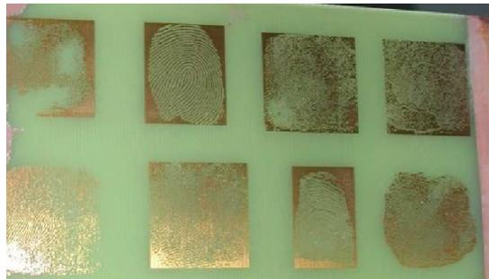
Figure 7: Finished PCB fingerprint mould.
