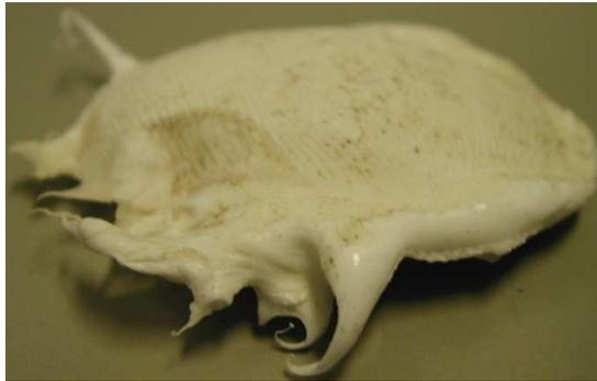
Figure 3: A working silicone finger, which was cast in a clay mould.
